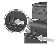
2 Pull the Punch Kit Release Lever [FS2] in the arrow direction, and open the Punch Kit.
