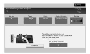
Return the original or paper, and tap [OK] or [Complete]; the system restarts scanning or printing of the original.
