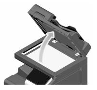
2 Wipe stains off the Slit Scan Glass using a dry, clean cloth.
