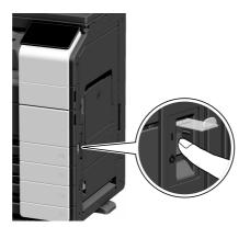
The **Power Indicator** on the **Control Panel** lights up, and the start screen is displayed on the **Touch Panel**.
